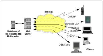
Figure 5. End-to-end transcoding generates multiple versions of a multimedia document prior to a client request. Each version is adapted for a specific client and/or access link. In response to a client request, the server returns the appropriate pre-transcoded version, thereby avoiding on-the-fly transcoding by a proxy.
