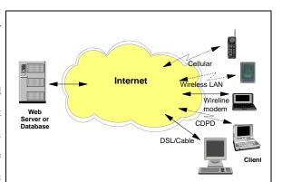
Figure 1. The emerging world of the wireless Web consists of a wide variety of fixed and mobile clients connected to the Internet over a wide range of link speeds, all trying to access multimedia content stored on a remote Web server or database.
