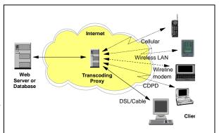
Figure 4. Proxy-based transcoding of multimedia content involves on-the-fly transformations of a server's content by an intermediate proxy for presentation to diverse clients connected to the Internet over diverse access links.
