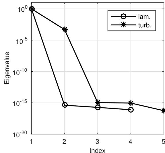
Figure 4. Normalized eigenvalues of  $\mathbf{C}$  for pipe flow study. A zero eigenvalue indicates that no change occurs along the associated direction. Note that the eigenvalues here imply that the laminar case has a 1D Active Subspace, while the turbulent case is two dimensional. Note that since the leading eigenvalue in the turbulent case is several orders of magnitude larger than the second, the first dimensionless parameter is more important – on average – than the second.
