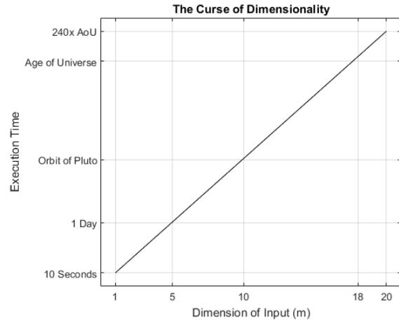
**Figure 1.** The computational cost of parameter studies increases exponentially with the dimensionality of the inputs; here we use a simple heuristic of sampling 10 points per dimension. If a computer code implementing  $f$  executes in one second, then the total execution time is  $10^m$  seconds. This quickly becomes infeasible for modestly large  $m$ .
