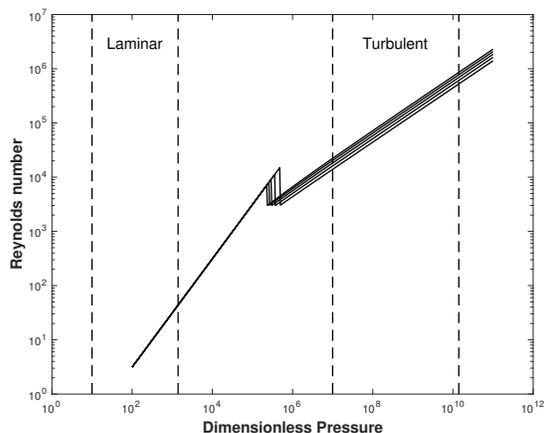
**Figure 3.** This diagram plots the Reynolds number against the dimensionless pressure. Different branches correspond to different values of Relative Roughness. Transition from laminar flow (Poiseuille relation) to turbulent flow (Colebrook equation) is assumed to begin at a critical Reynolds number of  $Re_c \approx 3 \times 10^3$ .
