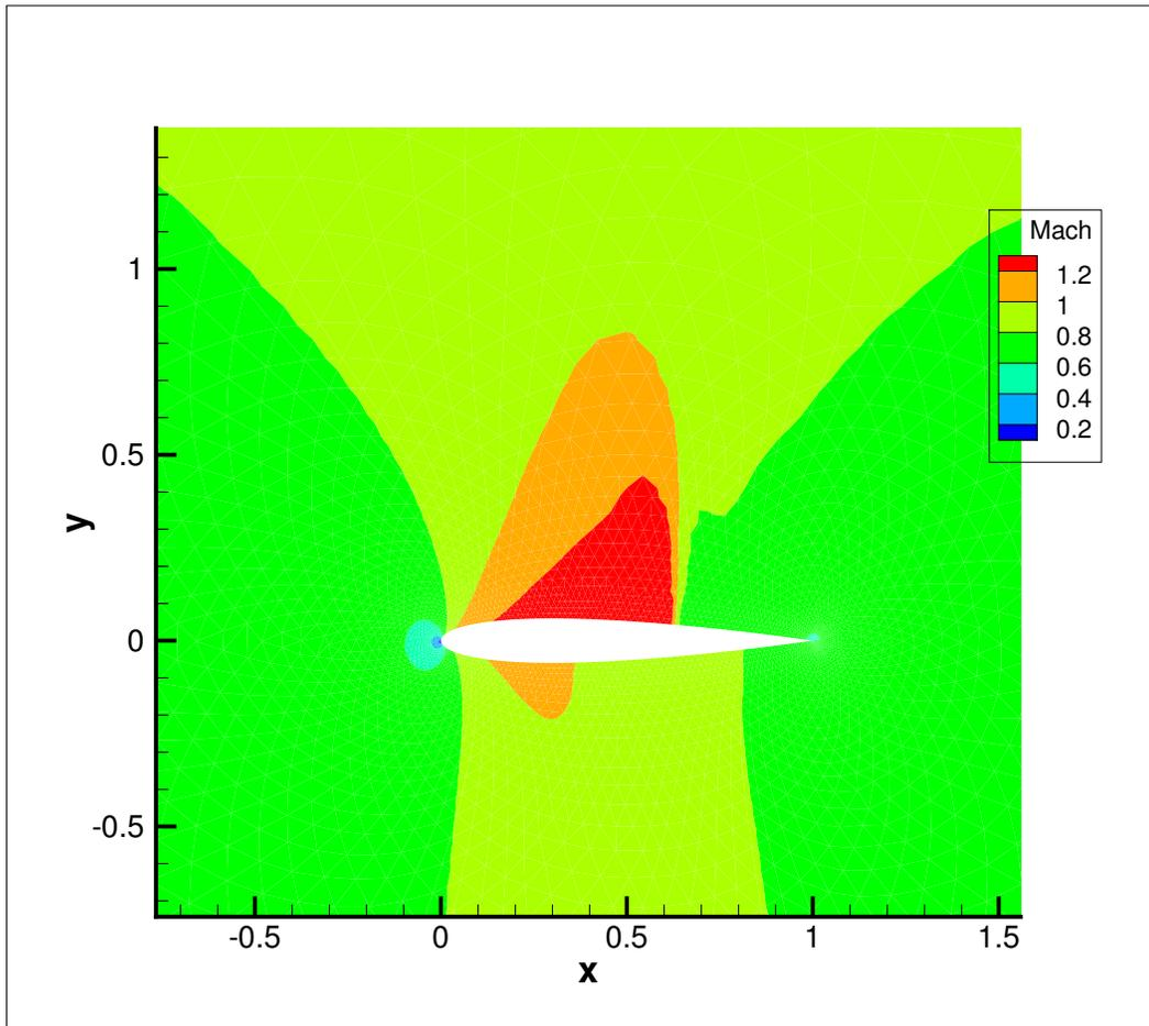
Figure 7. Inlet condition  $M_\infty = 0.8$ ; Mach contours over a NACA0012 airfoil.
