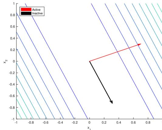
**Figure 2.** Active and Inactive directions for example function. Note that on average, the function changes more along the active directions than the inactive directions; in this case, the change in the inactive direction is exactly zero.
