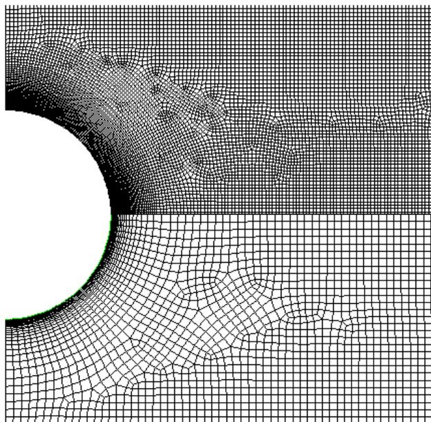
**Figure 2.** Unstructured grids used in the LES (top) and RANS (bottom) computations showing the strong clustering at the cylinder surface to capture the boundary layer.
