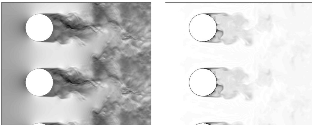
Figure 5. LES simulations. Instantaneous velocity (left) and temperature (right) contours for the turbulent flow around an array of cylinders.
