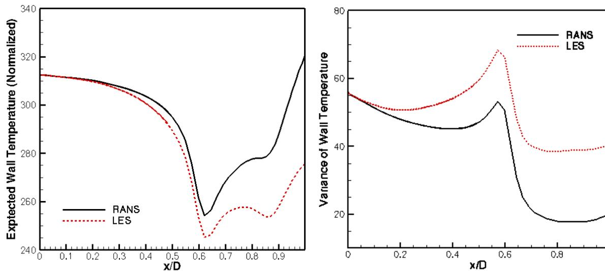
Figure 7. Temperature on the cylinder wall. Expectation (left) and variance (right) computed using RANS modeling and the LES technique. These calculations correspond to  $d_u = 2$ ,  $d_T = 1$ ,  $N = 13$  and  $M = 5$ .
