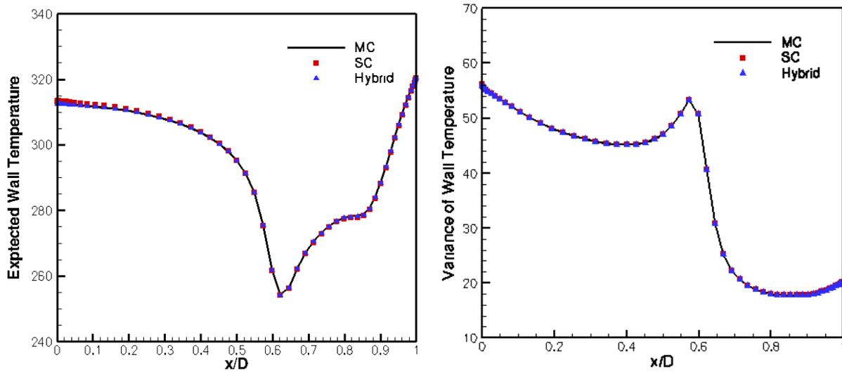
Figure 6. Temperature on the cylinder wall. Expectation (left) and variance (right) computed using RANS modeling and different uncertainty propagation methods. 1,000 samples are used in the Monte Carlo (MC) evaluation,  $N = 25$  evaluations are used in the stochastic collocation (SC) method and  $N = 13$  and  $M = 5$  are used in the hybrid method. These calculations correspond to  $d_u = 2$ ,  $d_T = 1$ .
