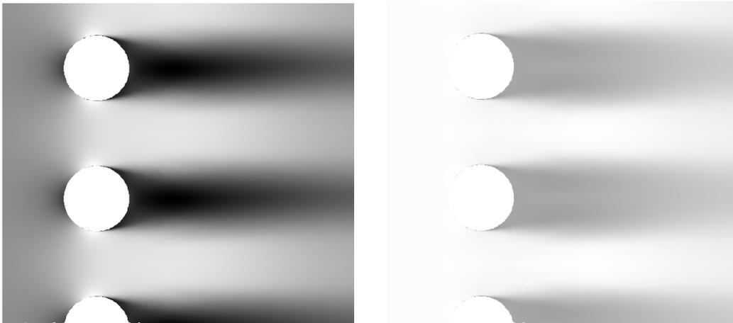
Figure 4. RANS simulations. Time-averaged velocity (left) and temperature (right) contours for the turbulent flow around an array of cylinders.
