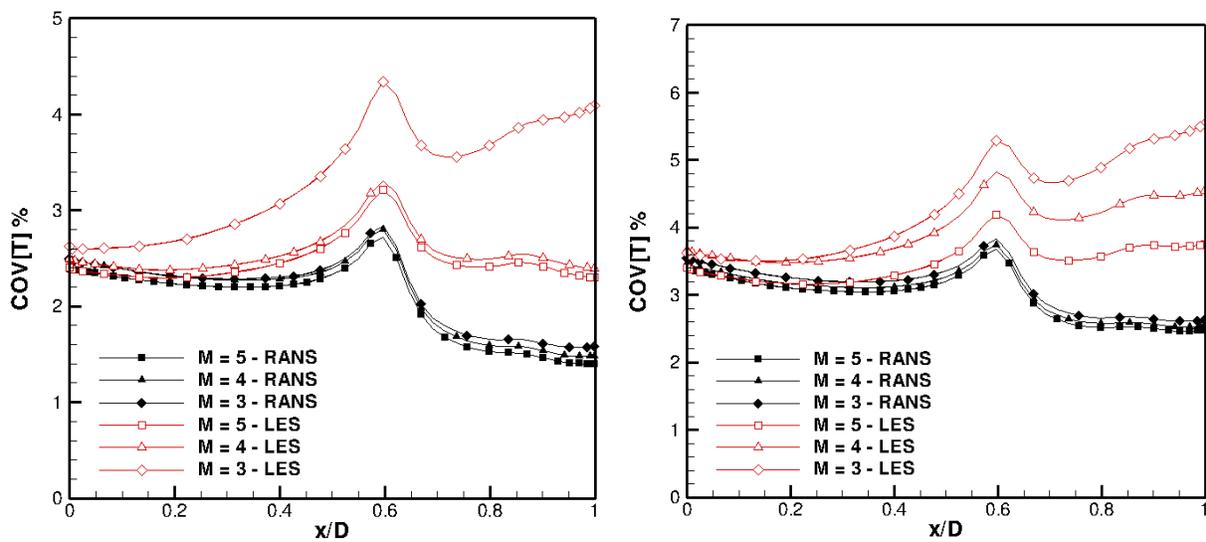
Figure 8. Coefficient of variation of the temperature on the cylinder wall. Effect of the order of the Galerkin expansion used for the energy equation for both RANS and LES modeling. The computations correspond to  $d_u = 2$  and  $d_T = 1$  (left) and  $d_u = 2$  and  $d_T = 2$  (right).
