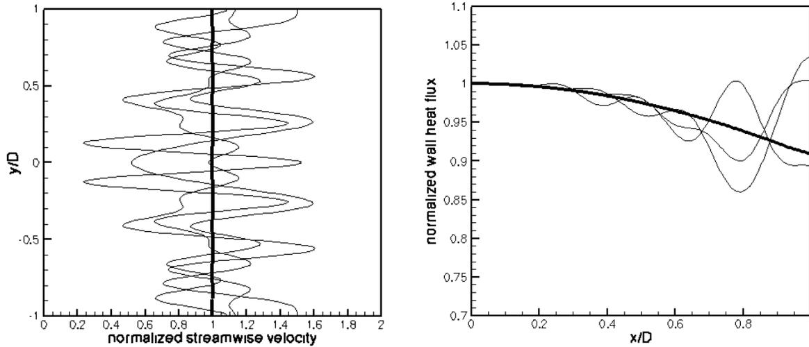
Figure 3. Inflow velocity (left) and wall heat flux (right) corresponding to three realizations (thin lines) and the expectation (thick line) from Eq. 13 and 14, respectively .
