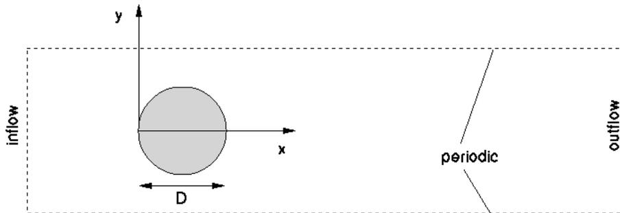
Figure 1. Sketch of the configuration used for the present numerical study.
