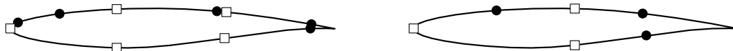
Figure 12. The location of the designed inspection points and uniformly spaced inspection points on the airfoil. Left: \lambda = 0.05 ; right: \lambda = 0.20 .
