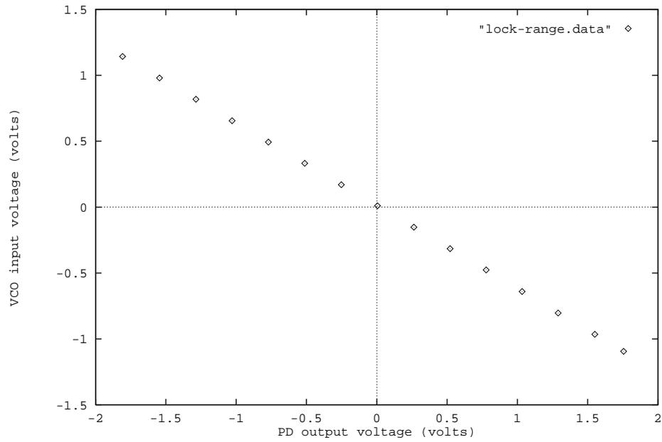
Figure 3: Locus of measured equilibrium states in locked loop: VCO input voltage versus PD output voltage
