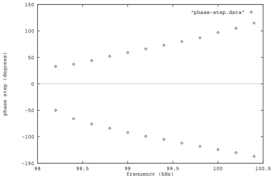
Figure 8: The maximum phase step that a locked loop can withstand, as a function of frequency. The edge of the lock range is 98.1kHz and the edge of the capture range is 100.8kHz
