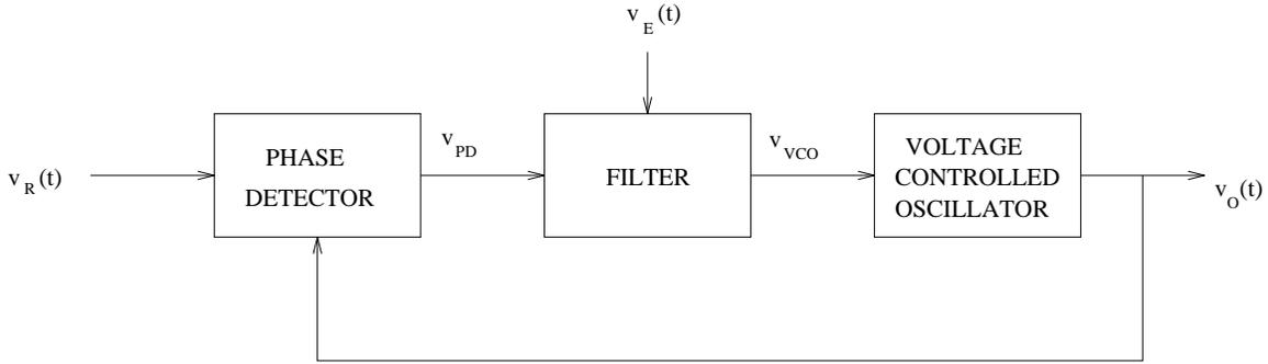
Figure 1: Phase-locked loop block diagram
