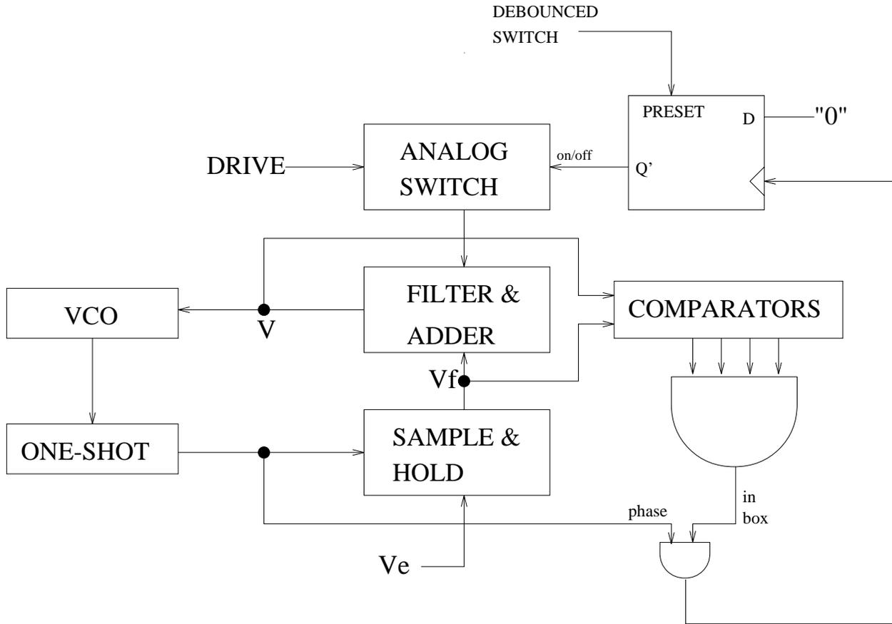
Figure 9: Block diagram of the phase-locked loop
