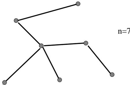
...the resulting *rigid body* only has six degrees of freedom: three for position and three for orientation. The rods act as *constraints* that reduce the dimension of the system, and the dynamics of the rotation/translation of the object are governed by a set of six second-order ODEs.
