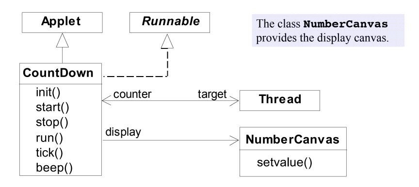
The class **CountDown** derives from **Applet** and contains the implementation of the **run()** method which is required by **Thread**.
