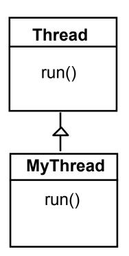
The Thread class executes instructions from its method run(). The actual code executed depends on the implementation provided for run() in a derived class.
