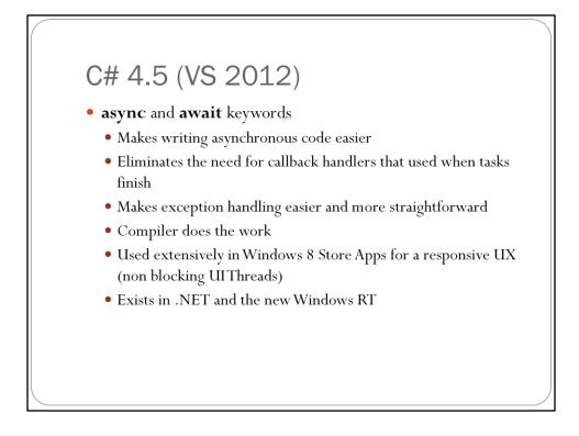
The goal of the Async and Wait keywords is to make asynchronous programming easier.
