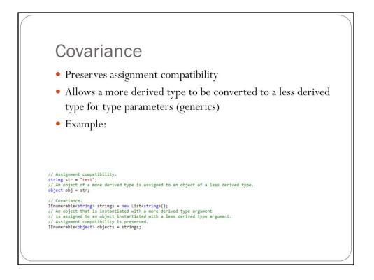
Covariance is sort of the opposite of Contravarience. It's used in generics where type parameters are passed. If you have a generic with a type parameter that is less derived from the one used then assignment compatibility is preserved. In the example above, the type *object*, which the most basic type is used to create a list of objects. But a list of *strings* is passed in that list of objects. Even though string is a more derived type, it works.
