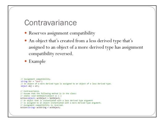
Contravarience allows a less derived type to be used as a type parameter in a delegate.
