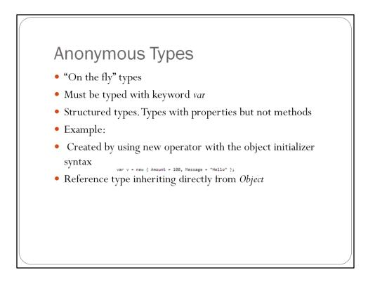
Anonymous types are used throughout the language for different reasons. It's mostly used by LINQ. It's a way to save a lot of code by not having to create a concrete type when you only need a type to temporarily by used to hold a few properties.
