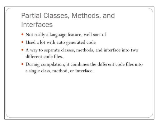
This is used extensively when the IDE creates a lot of auto generated code. You would create a partial class, method, or interface when you need to "hang" something off the auto generated code. Two common examples are designer classes where you have a WYSIWYG tool that generates code in the background and a ORM Tool that might generated a lot of classes based on the database design.
