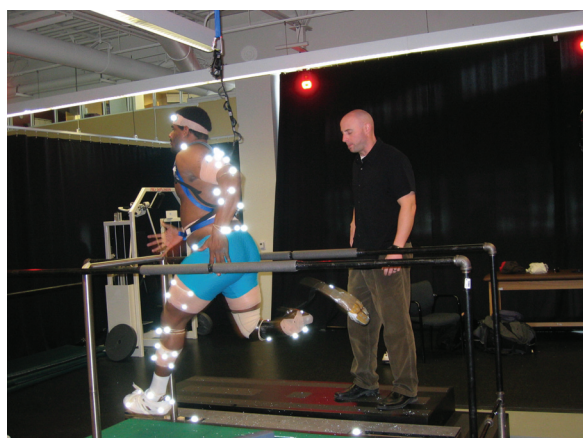
FIG. 1. Subject with a unilateral transtibial amputation running on a high-speed instrumented treadmill.
