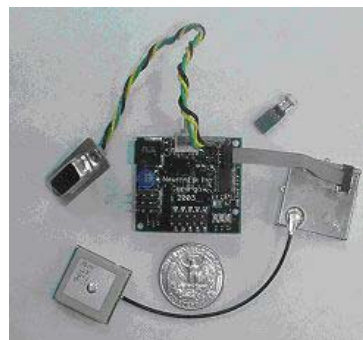
Figure 10: MANTIS nymph micro sensor node.
