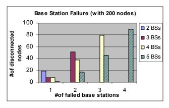
Figure 6 Effect of base station failure
