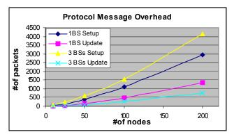
Figure 8 Number of packets exchanged during a base station relocation
