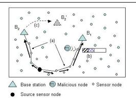
**Figure 1.** a) Multiple paths to multiple base stations b) disguising header address fields c) relocation of base station.
