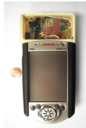
Figure 7: The MiniBrick and COMPAQ iPAQ are integrated together into a single package to form the UCOM Client Device.
