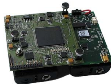
Figure 3. Custom sensor board and Mica2 mote.
