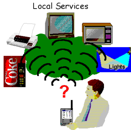
Figure 2. The active device resolution problem: Given N devices capable of being controlled, which user interface is the best candidate for being automatically pre-fetched into the user's remote control, so that the user can avoid manual selection before each remote control interaction?
