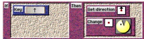
Figure 5. Rule: if cursor-up key is pressed, set new direction to up and change depiction to pacman facing up
