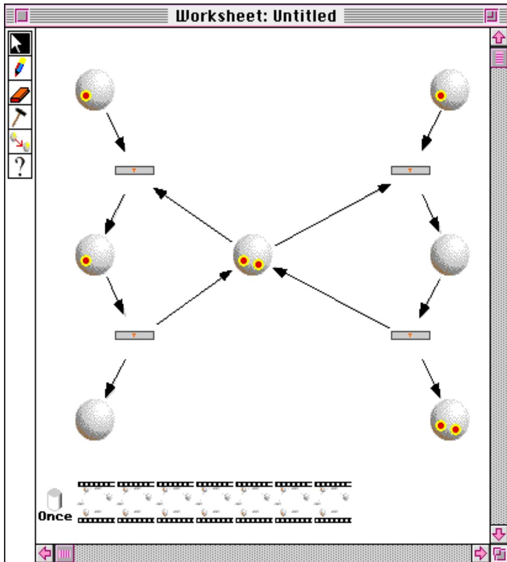
**Figure 29: Petri Net modeling two Processes sharing one Resource**
