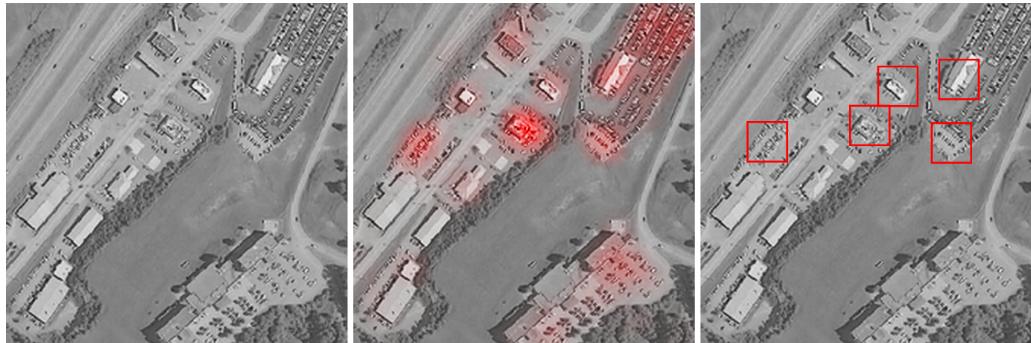
Fig. 1. (left) satellite image of an urban area; (middle) soft highlighting, where the saturation indicates the likelihood of a target; (right) hard highlighting, where a box is drawn around regions highly likely to contain a target
