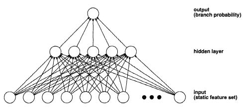
Figure 1: The branch prediction neural network. Each circle represents a processing unit in the network, and the links between units depict the flow of activity.
