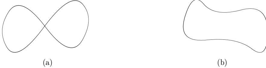
Figure 6: A closed curve in 3D, viewed from (a) the top and (b) the side. The latter projection is topologically conjugate to a circle; because of the self-intersection, the projection in (a) is not.
