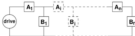
Fig. 16. The `xmission-line` meta-domain allows PRET to use its lumped-element GPN components to model spatially distributed systems like transmission lines, vibrating strings, and so on. The basic paradigm is an iterative structure with a variable number of sections, each of which has the same topology—a series element  $A_i$  and a parallel element  $B_i$ . The number of sections, each of which models a small piece of the continuum physics, rises with the precision of the model.
