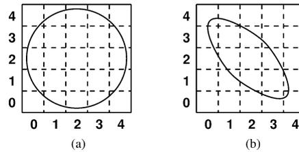
Fig. 7. Identifying a *period-one limit cycle* using the cell-dynamics method.
