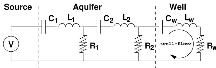
Fig. 18. PRET's model of the well/aquifer system of Fig. 15. The drive,  $V = d_a \sin d_f t$ , simulates a sinusoidal pressure fluctuation in the aquifer. Note how the GPN components let the load (the well) be incorporated naturally into the model.
