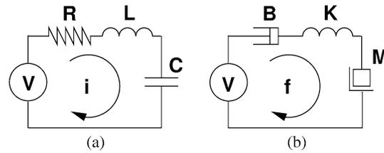
Fig. 4. Two systems that are described by the same GPN model: (a) a series RLC circuit and (b) a series damper-spring-mass system.  $V$  is a voltage source in (a) and a velocity source in (b).
