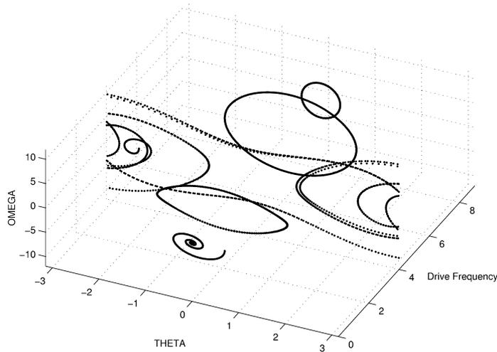
Fig. 8. The state/parameter (S/P) space portrait of the driven pendulum: a parameterized collection of phase portraits of the device at various drive frequencies. Each  $(\theta, \omega)$  slice of this S/P-space portrait is a standard state-space plot at one parameter value.
