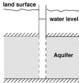
Fig. 15. An idealized representation of an open well penetrating an artesian aquifer. If the pressure in the aquifer fluctuates, the water level in the well will move in response.
