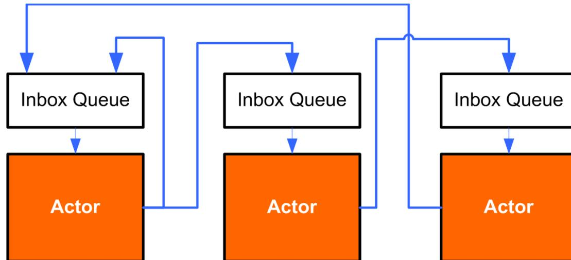
Fig: Message passing between objects, each object has an inbox (a queue) of messages which it works through and objects send messages to the inbox of other objects, where messages are immutable
