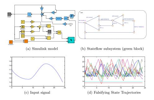
Fig. 2. Room heating benchmark HEAT30 and results obtained from S-TALIRO run.3 Usage
