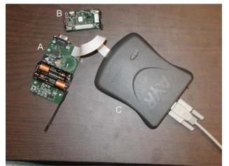
Figure 1) A) Programming board with Mica2 plugged in. B) Other side of Mica2. C) AVR ICE JTAG programmer connected to programming board with ribbon and connected to computer via serial cable.
