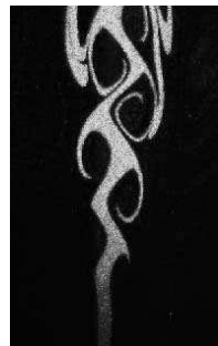
Figure 3.2: A planar air jet. Reynolds number \approx 70 . Synthetic jet actuator on one side at 1.94 KHz, modulated at 10 Hz. Vortices are clearly visible in this photograph of the jet.
