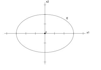
**Fig.1.** Ellipse  $\frac{x_1^2}{9} + \frac{x_2^2}{4} = 1$ ; equivalently center  $\mathbf{c} = \mathbf{0}$ ,  $\mathbf{B} = \begin{bmatrix} 9 & 0 \\ 0 & 4 \end{bmatrix}$ .
