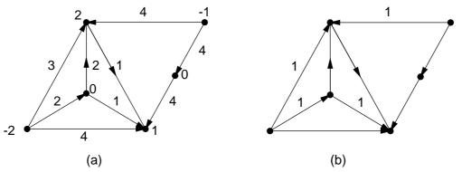
**Fig.2.** (a) Graph G with vertex demands & edge costs. (b) Optimum transshipment, cost 10. Edge labels give # units shipped on the edge; 0 labels are omitted. 1 unit is shipped along path 5,3,6 – vertex 3 functions as a transshipment node.
