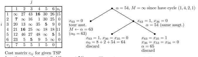
Cost matrix  $c_{ij}$  for given TSP & optimum assignment (boldface; cost 54) & optimum duals  $u_i, v_j$  (sum 54)
