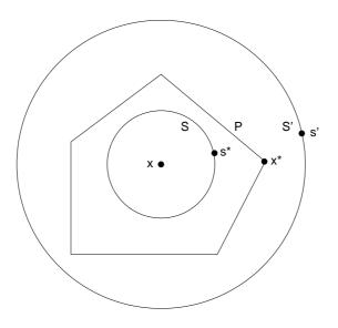
to make this precise suppose we're currently at point  $\mathbf{x}$  in the feasible region P let S(S') be balls contained in (containing) P with center  $\mathbf{x}$  let the radius of S' be  $\rho$  times that of  $S, \rho \geq 1$  let  $\mathbf{x}^*$  ( $\mathbf{s}^*, \mathbf{s}'$ ) have minimum cost in P(S, S') respectively
