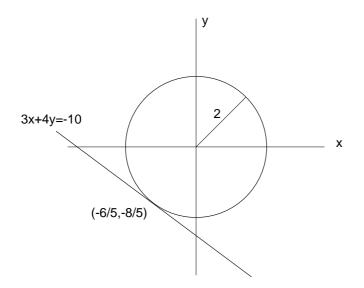
To minimize 3x + 4y over the disc with center (0,0) and radius 2 start at the center & move 2 units along (-3, -4) to (-6/5, -8/5)
